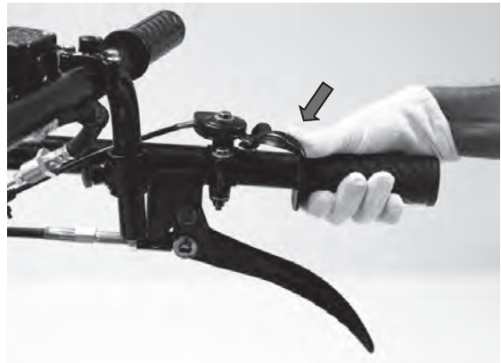
To increase engine RPM (fig-2)
