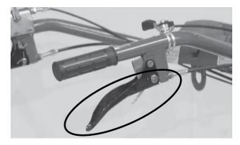
To operate the reverse lever, reverse lock should be pressed along with reverse lever to operate in reverse gear
