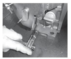
Drain the old / used oil and collect it in a container while the engine is warm to assure rapid and complete draining.
