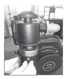
Step 5 - Reinstall oil bath bowl & tighten filter bowl clamps.
