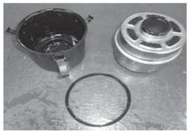
Step 4 - Clean Filter elements with diesel or kerosene & reinstall. If filter elements are damaged, replace with new one.
