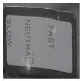
Reverse speed lever with reverse lock located on right hand side of handlebar with identification sticker
