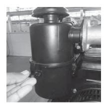
Step 1 - Loosen air filter clamps, separate oil bath bowl & filter element
