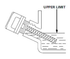
Reinstall oil filler cap & tighten.
