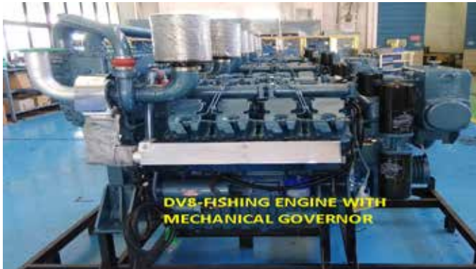
DV8 and DV 10 engines developed with Mechanical Governor. Seeding of 4 X DV 8 done in March 19.
